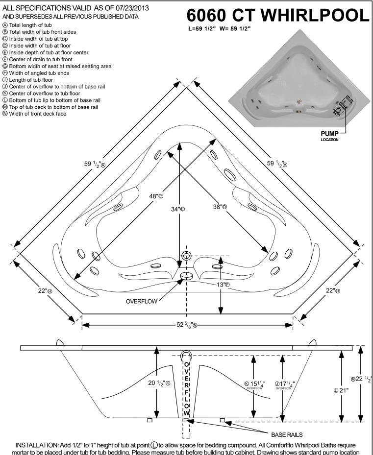
mortar to be placed under tub for tub bedding. Please measure tub before building tub cabinet. Drawing shows standard pump location for this tub. Custom pump locations available - please call Comfortflo Whirlpool Baths for details. Measurements are plus or minus 1/2", and are subject to change without notice. Filling this tub to the maximum may require an above average size or dedicated water heater. This data sheet supersedes all specifications published prior to this publication date.
